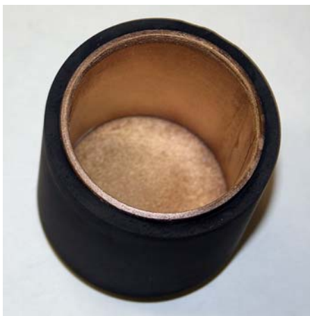
Fig. 1 63 mm diameter TaC crucible converted in situ from Ta metal. The TaC is gold colour whereas Ta is dark grey.
